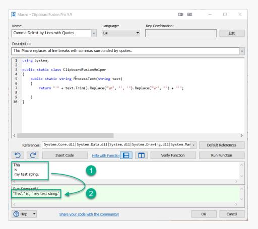
When clicking "Run Function" on successfully-written code, the input text entered in the input window (1) will be processed by the Macro functions, displaying the sample output along with "Run Successful" (2).
